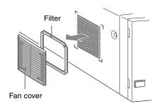
Clean the filter using the vacuum cleaner and the like.
